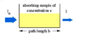
The Beer-Lambert law (or Beer's law) state that, when a monochromatic light pass through a solution, absorbance (A) of the solution is directly proportional to the concentration(c) of the solution and path length (b) that solution. Now absorbance A is directly proportional to path length and concentration of that solution.
