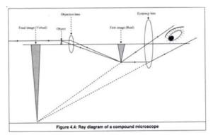
The objective lens produces a magnified 'real image' first image) of the object. This image is again magnified by the ocular lens (eyepiece) to obtain a magnified 'virtual image' (final image), which can be seen by eye through the eyepiece. As light passes directly from the source to the eye through the two lenses, the field of vision is brightly illuminated. That is why; it is a bright-field microscope.
