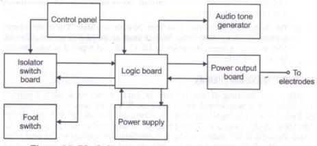
Figure 6.2: Block diagram of electrosurgical diathermy unit
