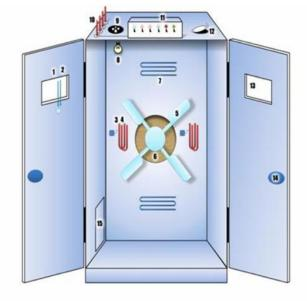
1. Wet-bulb Thermometer8. Work Light2. Dry-bulb Thermometer9. Air Cool3. Primary Heater10. Contact Thermometers4. Secondary Heater11. Control Panel5. Fan12. Air Outlet6. Gunny Curtain13. Glass Window7. Water Cooler14. Lock15. Side Door
