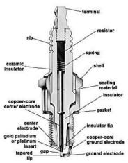
The above figures show clearly the construction of a spark plug. The plug has three main parts, the centre electrode, the ground electrode and the insulator separating them. Besides these,
