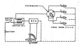
The workings of the basic distributor type electronic system is similar to the conventional electrical ignition system, except that in the electronic ignition system a timer is employed in the distributor instead of contact breaker. This timer may be a pulse generator or a Hall-effect
