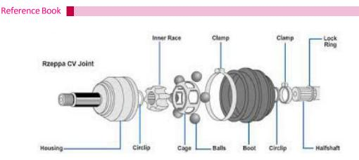
As shown in the figure, the joint consists of an outer race, inner race, cage and six balls. The joint can also slide in the axial direction on account of the balls sliding in the axial grooves of the outer race. Thus the drive shafts can accommodate the changes in their lengths.
