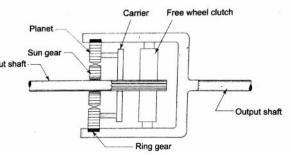
carrier can move on the splines on the input shaft. A free wheel clutch is also fitted on the input shaft splines. The output shaft is connected to the ring.
