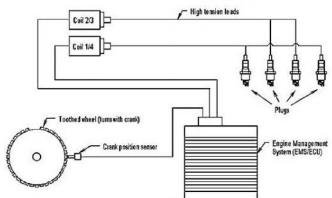
the waste cylinder. When the coil discharges, both plugs fire at the same time to complete the series circuit.
