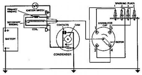
Note that the figure shows the ignition system for a 4-cylinder petrol enginethere are 4-spark plugs and contact breaker cam has 4-corners. (If it is for 6cylinder engine it will have 6-spark plugs and contact breaker cam will be a perfect hexagon).
