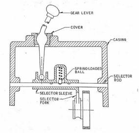
Figure shows a typical selector mechanism for a 4 forward speeds and one reverse gear box. The gear lever is ball mounted in the gear box cover. This facilitates its movement in any direction. The lower end of the gear lever fits into a slot in the selector sleeve. There are forks mounted on the sleeves on three separate selector rods which are supported in the gear box casing. Each selector sleeve
