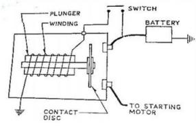
It is also called magnetic switch. As the button is pressed, the current flows from the battery to the winding which produces a magnetic field, resulting in the movement of the plunger to close the switch connecting the battery and the starting motor. The
