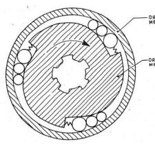
When the driving member is rotating in the direction as shown in the figure, the driven member will also be rotating in the same direction. But when the driven member becomes the driving member, the inner member will not rotate along with the outer one. Thus in this case the transmission and engine will be isolated from the wheels. This results in fuel economy.
