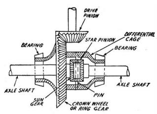
When the vehicle is going straight the cage and the inner gears rotate as a single unit and the two half shafts revolve at the same speed. In this situation, there is no relative movement among the various differential gears. To understand what happens when the vehicle is taking a turn, assume that the cage is
