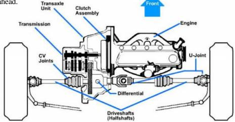
The operation of any transaxle is exactly the same as that of any transmission. The difference is this, instead of being connected via a long driveshaft to the rear axle, the transmission's output shaft drives a large gear that meshes directly with the
