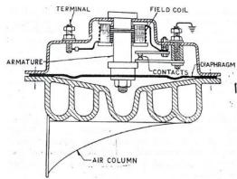
which is the position when the horn switch is in the off position. When the driver pushes the horn switch, the circuit is completed and the field coil produces an e.m.f. which causes the armature and along with it the diaphragm, to move down.
