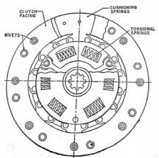
first has to compress the spring segments to flat condition resulting in smoother engagement.
