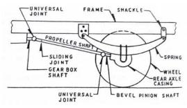
This is the simplest and most widely used type of rear axle drive. In this case the springs besides taking weight of the body, also take the torque reaction, driving thrust and the side thrust. The figure alongside shows such a drive. The propeller shaft is provided with two universal
