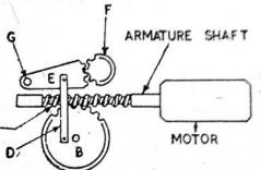
G. This motion is then imparted to a similar sector F on the spindle on which is mounted the wiper arm. Wiper blade is attached to the wiper arm by means of a spring lock. A rubber wiping element is held in place in the wiper blade. Wiper arms pivot against the windscreen under spring pressure to ensure adequate wiper blade pressure against the glass.
