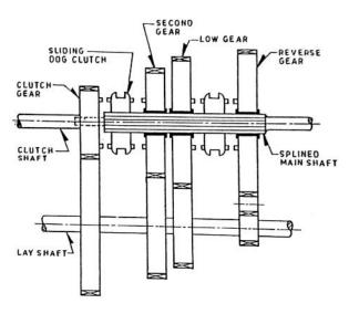
In this type of gear box, all the gears on the main shaft are in constant mesh with the corresponding gear on the lay shaft. The gears on the main shaft, which is splined, are free. The dog clutches are provided which are free to slide on the main shaft. The gears on the lay shaft are fixed.
