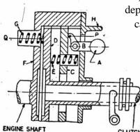
is required. The clutch is operated automatically depending upon the engine speed. This means that car can be stopped in gear without stalling the engine. Similarly while starting, the driver can first select the gear, put the car into the gear and simply press the accelerator pedal. This makes driving very comfortable and easy.
