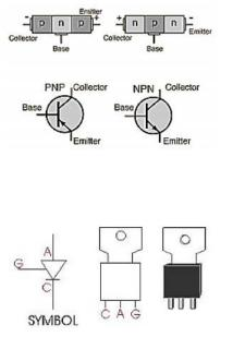
current ratings from a few amperes to very nearly thousand amperes. The family of thyristors consists of PNPN diode (Shockley Diode), SCR, LASCR, TRIAC, DIAC, UJT etc.
