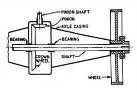
The figure shows a simplified view of the live rear axle of a front engine, rear driven automobile. The differential is not shown purposely, so as to make the general arrangement more clear. The drive from the propeller shaft comes to the pinion shaft which is supported in bearings in the axle casing. The
