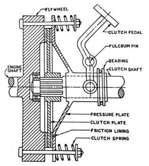
When the clutch pedal is pressed the pressure plate is moved to the right against the force of springs. This is achieved by means of a suitable linkage and a thrust bearing. With this movement of the pressure plate the friction plate is released and the clutch is disengaged.
