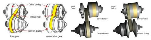
The CVT replaces the gears with two variable-diameter pulleys, each shaped like a pair of opposing cones, with a metal belt or chain running between them. One pulley is connected to the engine (input shaft) and the other to the drive wheels (output shaft). The halves of each pulley are movable; as the pulley halves come closer together the belt is forced to ride higher on the pulley, effectively making the pulley's diameter larger.
