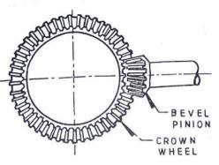
in contact. As a result an uneven transmission of motion will take place as the load is transferred from one pair of teeth to the next. Thus these gears are noisy and suffer from high wear.
