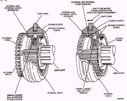
Synchromesh devices utilize a multi-plate clutch or a conical clutch to equalize the speeds of the input and the output rotating members of the gearbox during the process
