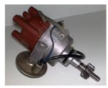
The distributor is rotated by the distributor shaft, which in turn is driven by the camshaft of the engine. The distributor has a rotor which rotates at half the speed of the engine crankshaft. The distributor itself rotates at the same speed as the camshaft.
