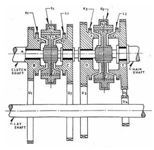
are to be engaged are first brought into frictional contact which equalizes their speed, after which these may be engaged smoothly.
