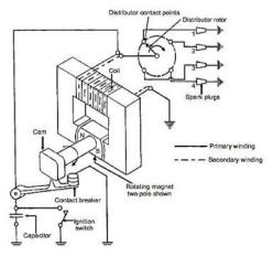
secondary windings rotate between the poles of a stationary magnet.
