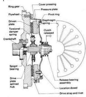
Diaphragm spring is supported on a fulcrum retaining ring so that any section through the spring can be regarded as a simple lever. The pressure plate is movable axially, but it is fixed radially with respect to cover. This is done by providing a series of equally spaced lugs cast upon the back surface of the pressure plate. The drive from engine flywheel the is transmitted through the cover, pressure plate and the friction plate to the gear box input shaft.
