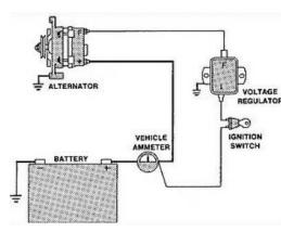
A typical charging system contains an alternator (generator), drive belt, battery, voltage regulator and the associated wiring. The charging system, like the starting system is a series circuit with the battery wired in parallel. After the engine is started and is running, the alternator takes over as the source of power and the battery then becomes part of the load on the charging system.
