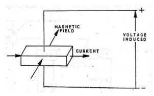
The principle of operation of this type of pulse generator is based on the Hall effect. When a chip made of semiconductor material carries a signal current across it and is exposed to a magnetic field, a small voltage called the Hall voltage is generated between the chip edges at 90 degrees to the path taken by the
