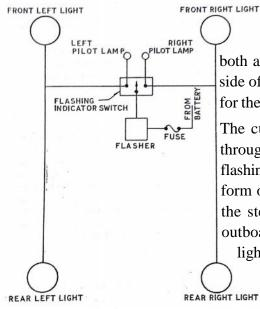
One light on each side is fitted both at the front as well as on the rear side of the vehicle. The wiring diagram for the same is shown in the figure.
