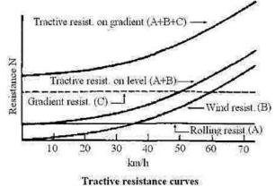
When a vehicle is travelling at constant speed, its resistance to motion is termed as the tractive resistance. Whenever the tractive effort exceeds the total Wind resist. (B) resistance, the vehicle will accelerate.
