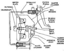
Hydraulic clutch activation systems consists of a master cylinder and a slave cylinder. When pressure is applied to the clutch pedal (the pedal is depressed), the pushrod contacts the plunger and pushes it up the bore of the master cylinder. During the first 1/32 in. (0.8 mm) of movement, the center valve seal closes the port to the fluid reservoir tank and as the plunger continues
