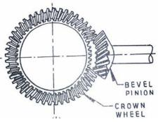
These types of gears are widely used for final drive these days. In this the pinion shaft is placed below the axis of the crown wheel. This permits a lower position of the propeller shaft, thus allowing low chassis height. The name 'hypoid' is derived from the 'hyperboloid of revolution'. The basic surface on which the teeth are cut in their case, is hyperboloid,
