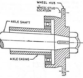
in the plane of the road wheel. However, it has to take the end loads and the driving torque.
