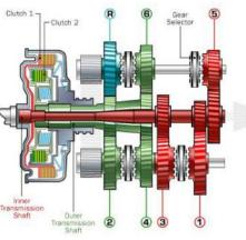
Schalt Getriebe" but it also has an English alternative of "Direct Shift Gearbox". The reason for such a naming is because two transmission systems are integrated into one. Transmission one includes the odd gears (first, third, fifth and reverse), while transmission two contains the even gears (second, fourth and sixth). The combined dual clutch system switches from one to the other very quickly, releasing an odd gear and at the same time engaging a preselected even gear
