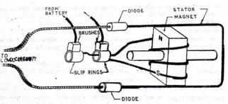
reverses its polarities; the current produced in the stator changes in sign in a revolution. To convert the alternating current into direct current; diodes pass through them only in one direction. Thus AC current is converted into DC current to supply power for various electrical needs.
