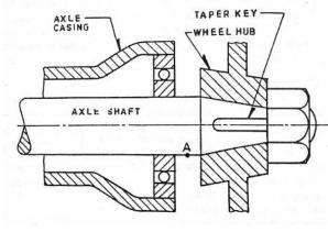
The figure shows a semi floating axle. The wheel hub is directly connected to the axle shaft or is an extension of the same. The inner end of the axle shaft is splined and is supported by the final drive unit, whereas the outer end is supported by a single bearing inside the axle casing. In this
