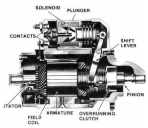
The overrunning clutch, which is employed in this type of drive is shown in the figure. It consists of a shell and a pinion collar connected in such a way that when the shell is rotating at a speed greater than that of the pinion collar, the former will drive the later. However, whenever the speed of the collar becomes more than the speed of the shell, there is no more connection between the two. Such
