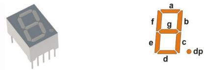
Here is how an optical illusion based on the same operating principle as a film camera is made. Only one digit at a time is active, but they change their state so quickly that one gets impression that all digits of a number are active simultaneously.
