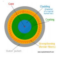
**cladding**, a glass or plastic coating that has optical properties different from those of the core.
