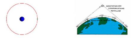
Communications satellites are often in geostationary orbit. At the high orbital altitude of 36,000 kilometers, a geostationary satellite orbits the Earth in the same amount of time it takes the Earth to revolve once. From Earth, therefore, the satellite appears to be stationary, always above the same area of the Earth. The area to which it can transmit is called a satellite's footprint
