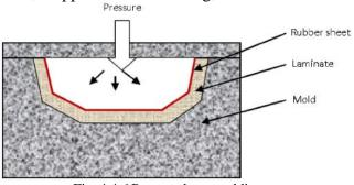
Fig: 4.4.6 Pressure bag moulding
