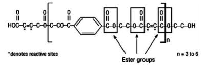
Fig: 4.3.3 Chemical structure of typical Isophthalic polyester
