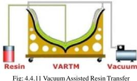
Aig: 4.4.11 Vacuum Assisted Resin Transfer Moulding
