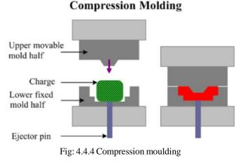
pre-cut to conform to the surface area of the mould.
