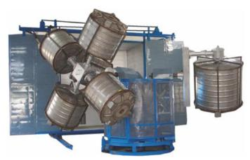
Fig: 3.4.5 Rotational Moulding machine
