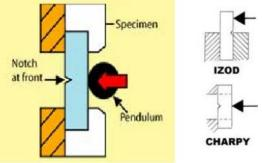
Fig: 3.6.4 Charpy impact testing
