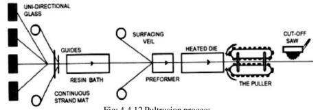
Fig: 4.4.12 Pultrusion process
