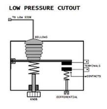
then the low pressure switch cuts off the compressor. Unlike the high pressure cut out, the low pressure cut out is self-resettable and does not need to be reset manually.
