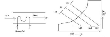
The bypass factor for the process is defined as the ratio of the difference between the mean surface temperature of the coil leaving the air temperature and the difference between the mean surface and the entering air temperature.
