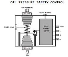
the electronic control, the pressure sensor sends a signal to the control module whenever the pressure sensed falls below 7 from 9 psig. This signal causes the control module to open the safety contact points after a time delay. This control also requires manual reset, once it is tripped. In both controls, the opening of the safety contacts breaks the electric current in the system control circuit.
