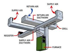
In air conditioning systems the 'duct' is considered a static component of the installation through which air flows within the building, connecting all parts of the system and via used or exhaust air is discharged.
