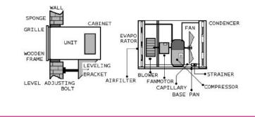
This type of AC is designed to fit into the window sills. A single unit of Window Air Conditioner houses all the necessary components, namely the compressor, condenser, expansion valve or coil, evaporator and cooling coil enclosed in a single box. Since the window AC is a single unit, it takes less effort to install as well as maintain.
