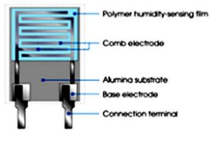
A thick film conductor of precious metals like gold, ruthenium oxide is printed and calcinated in the shape of the comb to form an electrode. Then a polymeric film is applied on the electrode; the film acts as a humidity sensing film due to the existence of movable ions. A change in impedance occurs due to the change in the number of movable ions.
