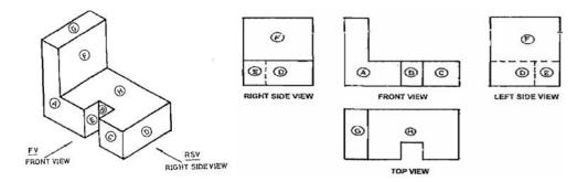
**Isometric projection:** The isometric projection of an object is a one plane view drawn with the object placed with respect to the plane of projection so that all the three principal axes appear to be inclined to each other at an equal angle of 120<sup>o</sup>.
