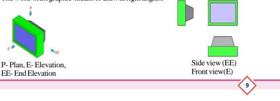
Basics of Orthographic Projection: Orthographic Projection helps us see an object in 2D. To do this we need to look at 90 degrees to the face of an object. The planes of projection are extended beyond the line of intersection to form four quadrants. The position of objects in any one of these four quadrants are as follows:
