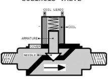
Their tasks are to shut off, release, dose, distribute or mix fluids. They are found in many application areas. Solenoids offer fast and safe switching, high reliability, long service life, good medium compatibility of the materials used, low control power and compact design. Besides the plunger-type actuator which is used most frequently, pivoted-armature actuators and rocker actuators are also used.
