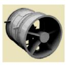
Vaneaxial fans are similar to tubeaxials, but with the addition of guide vanes that improve efficiency by directing and straightening the flow. As a result, they have a higher static pressure with less dependence on the duct static pressure. Such fans are used generally for pressures upto 500 mmWC.
