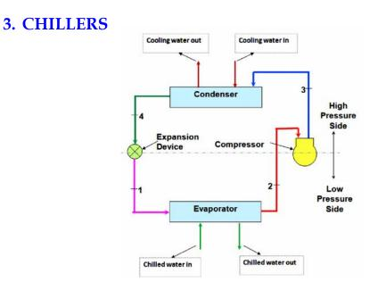
A *chiller* is a machine that removes heat from a liquid via vapour-compression or absorption refrigeration cycle. This liquid can then be circulated through a heat exchanger to cool air or equipment as required.
