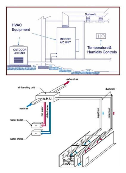
**Ductwork** is a branching network of round or rectangular tubes. It is generally constructed of sheet metal, fiberglass board, or a flexible plastic and wire composite material and is located within the walls, floors, and ceilings of the building.
