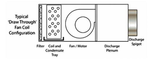
FCU is the abbreviation used for FAN COIL UNIT that are available for either DX or chilled water system that houses refrigerant or chilled water coil respectively. Beside the type of coil used, the other components are common such as the blower fan & filters. FCUs are usually available from 0.75 to 5 TR from various brands across the globe.
