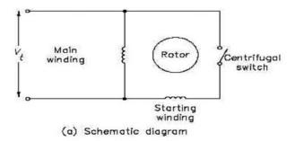
Split phase induction motors have two windings, starting and main windings. The starting winding is made of thinner wire and fewer number of turns than the main winding. At the time of starting, due to phase difference, high starting torque is produced and the motor starts to rotate. When motor reaches 70 to 80 % of its speed the centrifugal switch disconnects the starting winding from the circuit. Application: Refrigerator
