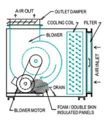
AHU. The purpose of this equipment is to collect and mix outdoor air with that returning from the building space. The air mixture is then cooled or heated, after which it is discharged into the building space through a duct system made up of five-feet diameter pipes. Air Handler is normally associated with heating/cooling (HVAC) systems in commercial buildings. These are normally very large systems moving from 2000 CFM to 10,000 CFM and higher. They may be mounted on the top of
