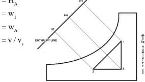
Sensible heat gain due to in filtered air  $= m (H_A - H_2)$ Latent heat gain due to in filtered air  $= m (H_1 - H_A)$ Ventilation required per person
