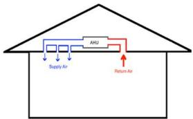
**SUPPLY DUCT CONFIGURATIONS** The configuration of a duct system is often like a tree with branches connected to the terminal units and a fan located at the root. In reality, the ductwork forms a double tree because the fan is in the middle of the supply and return/outside air parts of the system. The two most common supply duct systems are the 'extended plenum' system and the 'radial' system because of their versatility, performance, and economy.
